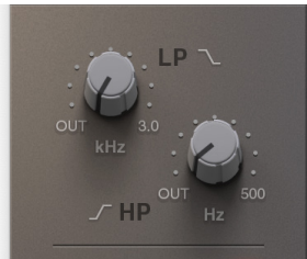
Low and High Pass Filters
