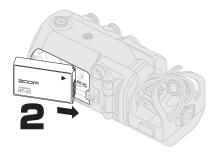
Install the rechargeable battery and close the battery cover.
