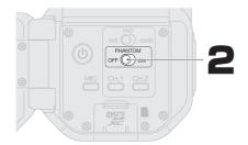
Set the PHANTOM switch according to the connected mic(s).
