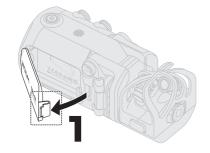
While pressing the latch, open the battery cover.
