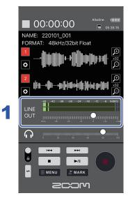
1. Slide the LINE OUT volume control on the Home Screen left and right to adjust the level.
