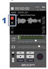
**1.** Tap the input selection buttons on the HOME screen for the inputs to record.
