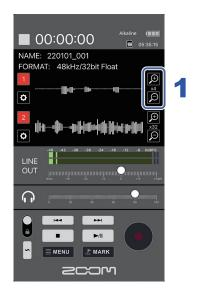
Adjust the input signal waveform to a size that is easy to check.
