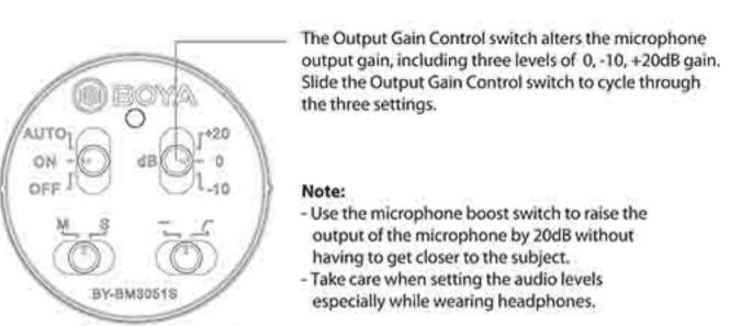
Slide the Output Gain Control switch to cycle through the three settings.
