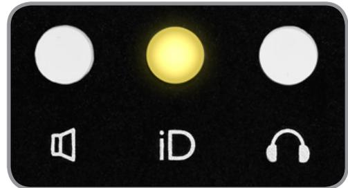
The iD button provides extra functionality in the form of an assignable function button, or it can be used to activate iD14's *ScrollControl* which turns the encoder into a virtual scroll wheel allowing you to control elements of your DAW ([see page 22](#))
