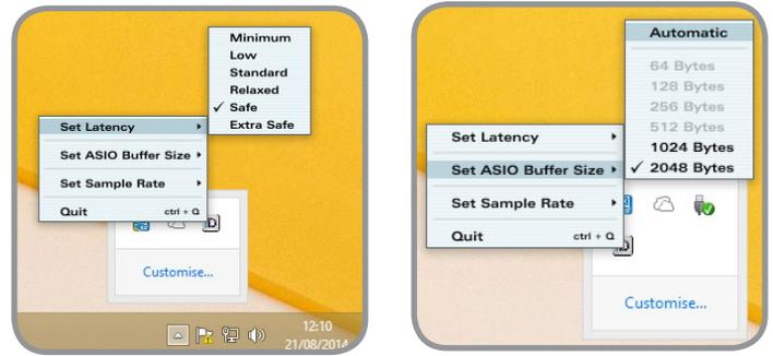
Latency refers to how often iD14 sends and receives its data, for example it is not possible to have a high latency setting and a low buffer size because the buffer would fill up with samples before iD14 has the chance to send them.
